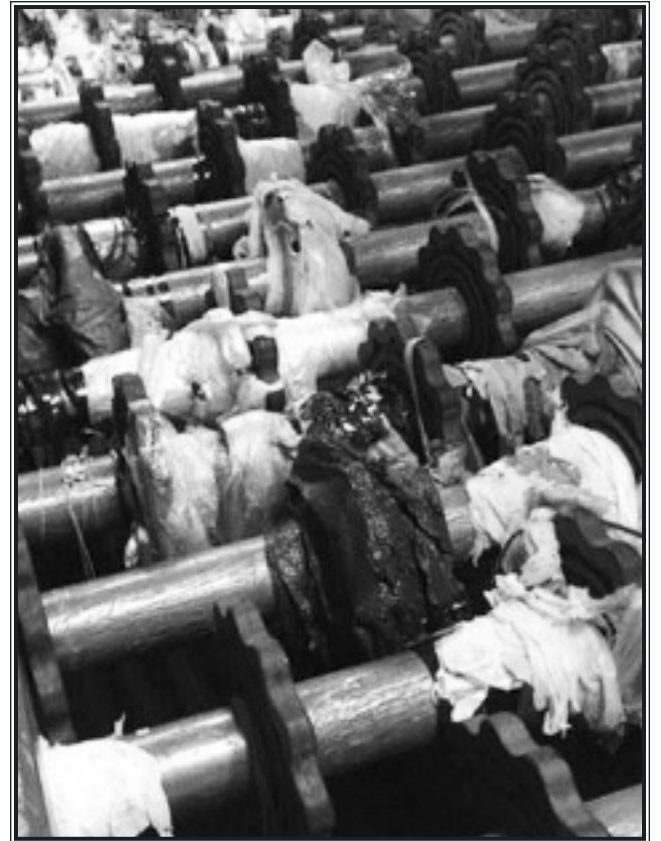
The town's recyclables are processed at a materials recovery facility (MRF) which gets clogged up and slowed down by plastic bags. Courtesy photo
